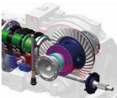
A computer aided design (CAD) – left – and computer-aided engineering (CAE) model of a gear box—right. Courtesy: PTC Creo (left) and ANSYS (right)
